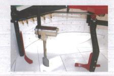
SICOMA -OMG Planetary Mixers can be equipped with a probe which is fixed to the scraping arm connection and rotates immersed in the mix for a faster and better measurement. A unique feature of our planetary mixers is
