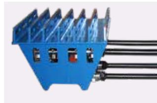
With the KVM variable vibration system it is possible to freely and independently adjust both frequency and amplitude during both the filling and compacting cycles. The vibration table bearings are oil lubricated giving long life and high serviceability.
