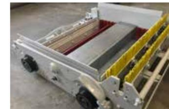
The unique KVM filling system is based on utilizing the correct type of filling box and controlling the amount of concrete delivered into the filling box. This ensures a precise filling and uniform product density, height and surface quality.
