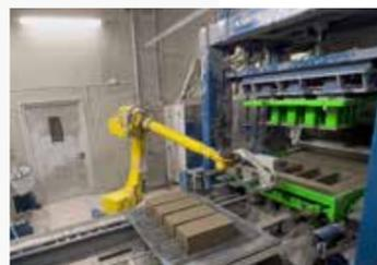
Robot systems implemented at the block machine's workstations replace a wide range of manual work tasks, heavy lifts and monotonous movements, thereby ensuring a good working environment for the operator and significantly reducing cycle time.
