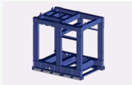
The main machine frame is a welded construction. Heavy plates are used to form a deep horizontal box under the whole machine to ensure optimum rigidity and fatigue resistance. This supports the RHS columns and vibration table. The machine is mounted on a sub frame isolated from the main frame by isolation dampers designed to absorb up to 95% of the vibrations.
