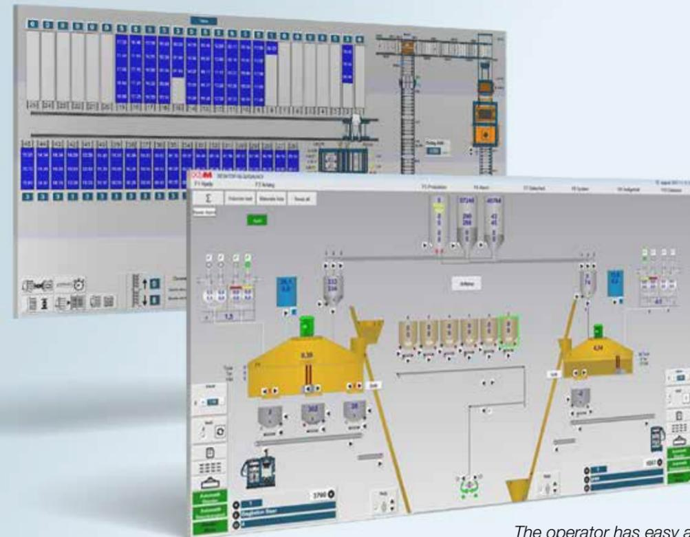
*The operator has easy access to all relevant production data giving an overview of the status of relevant parts of the entire plant.*
